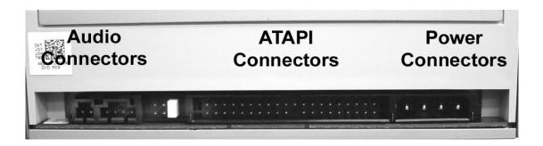
Power Connector Power is supplied to your DVD-ROM drive by the connection with your computer's +5V/+12V power cable to the power socket at the back of drive. One side of the plug has chamfered edges, so the power connector fits only one way
